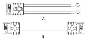
Anderson connector is used on the DC input side of wall mounted battery series. The specific connections are as follows:
